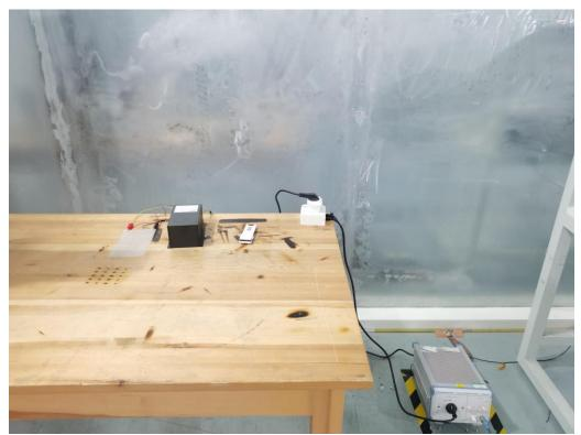
Photo of Power Line Conducted Measurement
