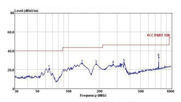
Freq Reading CabLos Antfac Measured Limit Over Remark dBuV dB dB/m dBuV/m dBuV/m MHz dB 65.11 9.53 0.52 10.66 20.71 40.00 -19.29 1 QP 2 135.98 17.31 0.70 8.49 26.50 43.50 -17.00QP 3 187.10 14.59 0.98 10.30 25.87 43.50 -17.63 QP 273.23 11.96 12.46 1.04 25.46 46.00 -20.54QP 5 349.25 11.97 1.13 14.26 27.36 46.00 -18.64QP 758.04 11.77 19.54 33.00 46.00 -13.00
