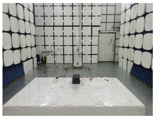
Photo of Radiated emission Measurement
